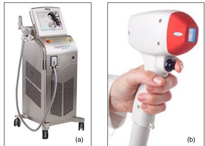
Figure 1. Alma Soprano ICE hair removal platform (a) and Alexandrite wavelength (755nm) based ALEX module (b)
